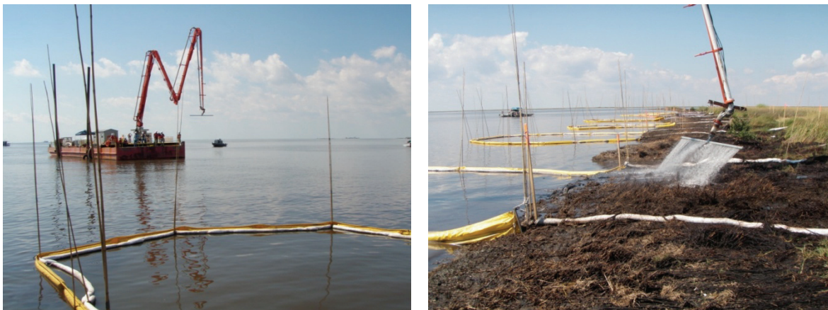
Figure 3-11. The barge-mounted flushing system that had a long-reach mechanical boom with a spray bar attached, Deepwater Horizon oil spill. The angle and pressure of the water spray had to be adjusted to minimize sediment erosion. However, this technique was not effective because the oil was too viscous to be flushed. Photo credit: Scott Zengel.
