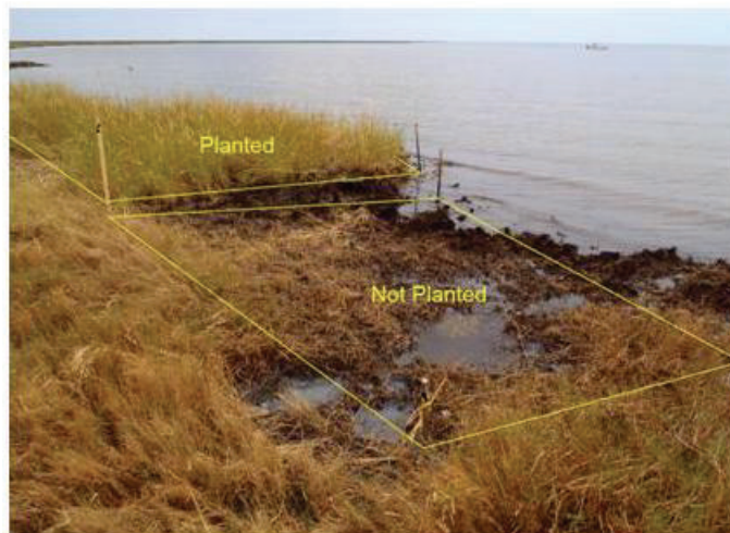
Figure 3-15. Tulane University research project where S. alterniflora was planted (bare root) along the heavily oiled and highly erosional shoreline in N. Barataria Bay, Louisiana, immediately following oil cleanup treatments. The treated and planted plot had good vegetative cover as of September 2012, whereas the treated but unvegetated plot had higher shoreline erosion. Photo credit: Scott Zengel.
