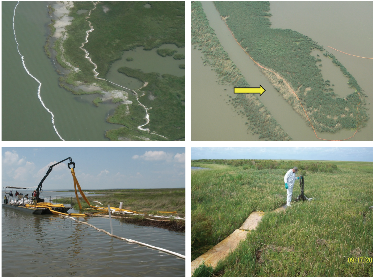
Figure 3-2. Top row: boom stranded on salt marshes (left) and Phragmites marsh in Louisiana in July 2010 after the passage of two storms that generated waves and high water. Photo credit: Andy Graham. Bottom row: specialized boom removal teams removed the stranded boom using various techniques to minimize further damage to the marshes. Photo credit: Deepwater Horizon Response.
